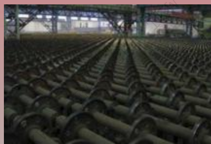
A large cooling bed for steel plates. Each wheel is supported by four high temperature bearings.
